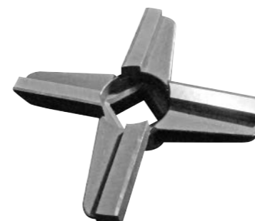
Bimetallic knife mod. "USA" with braze welded HSS inclined inserts mod. 32 - h 18,6 mm mod. 42 (52) - h 20 mm
